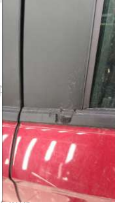
Sol arka cam fitili deformeler var
