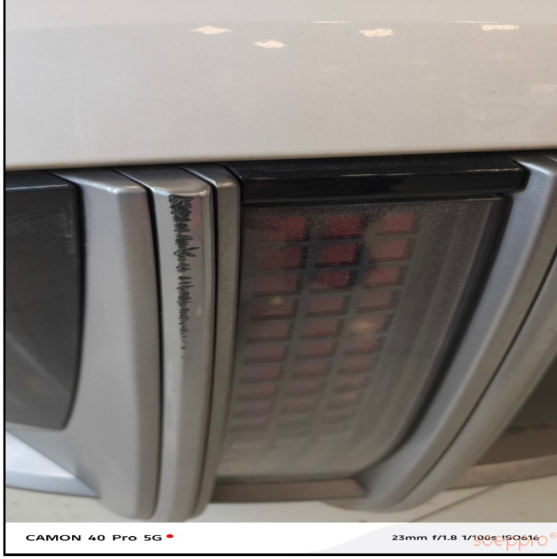
Arka tamponda deformeler var
