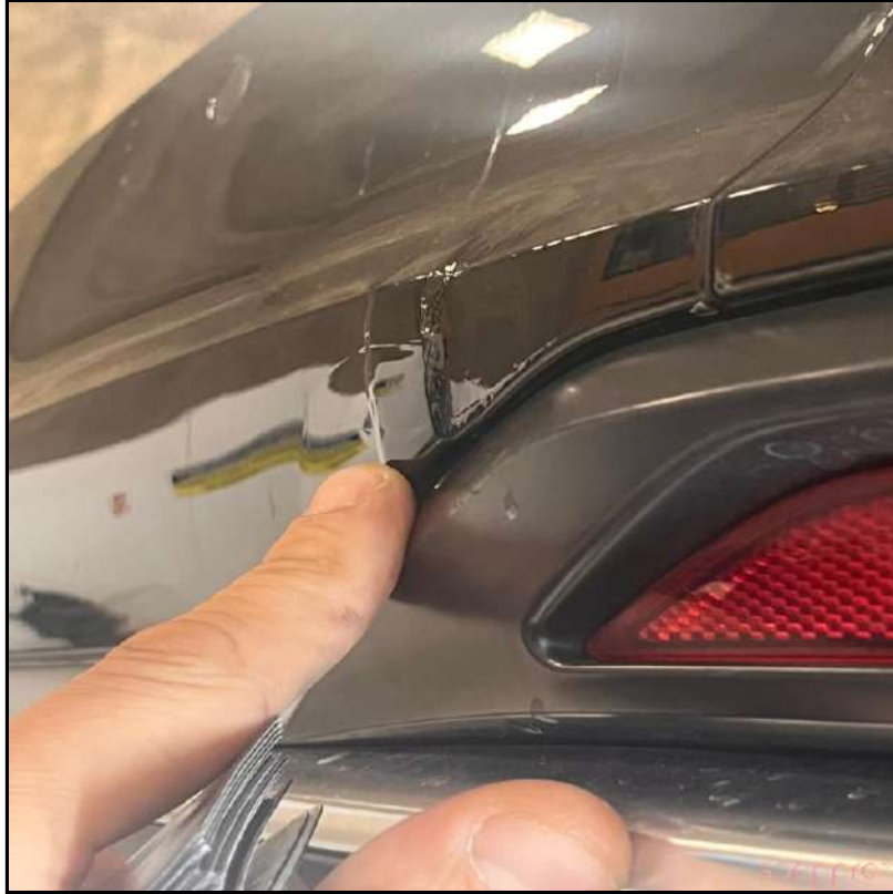
ARKA TAMPONDA DEFORMELER VAR
