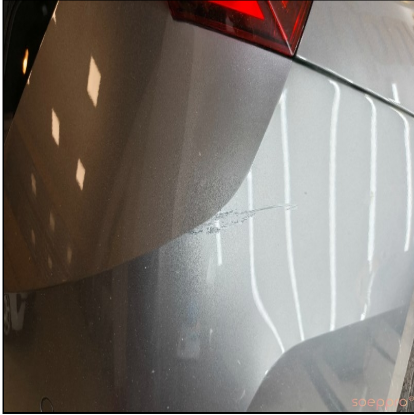
Arka tamponda deformeler var
