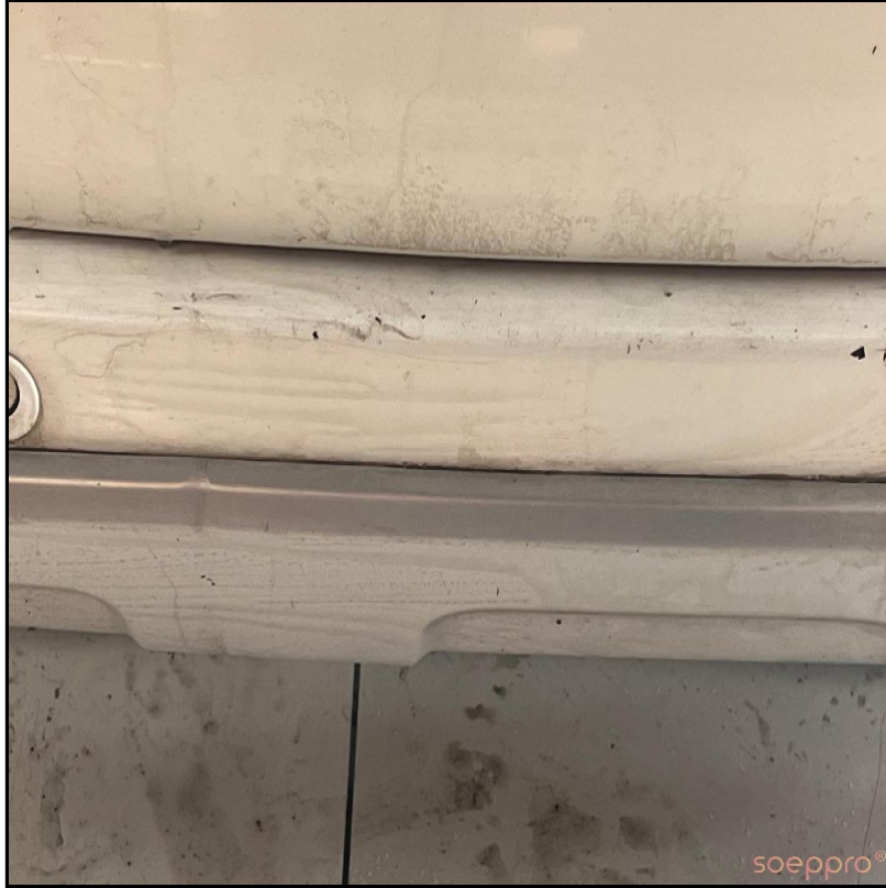
ARKA TAMPONDA DEFORMELER VAR
